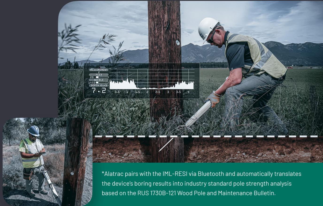
\*Alatrac pairs with the IML-RESI via Bluetooth and automatically translates the device's boring results into industry standard pole strength analysis based on the RUS 1730B-121 Wood Pole and Maintenance Bulletin.
